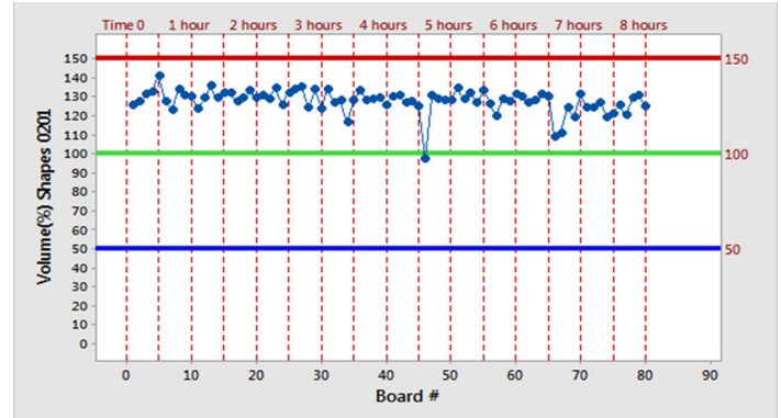
FIGURE 4. SPI values of solder volumes using AIM-recommended under-stencil cleaner.
