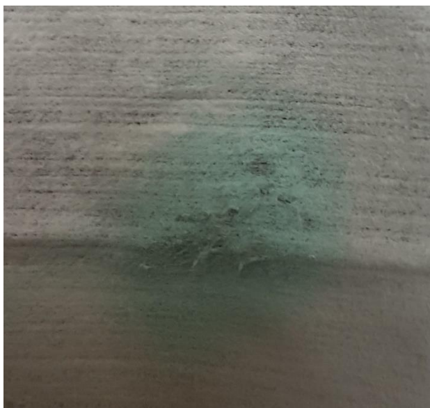
FIGURE 3. Greenish color deposited on a Solder Mask Check Wipe indicating a solder mask curing problem.
