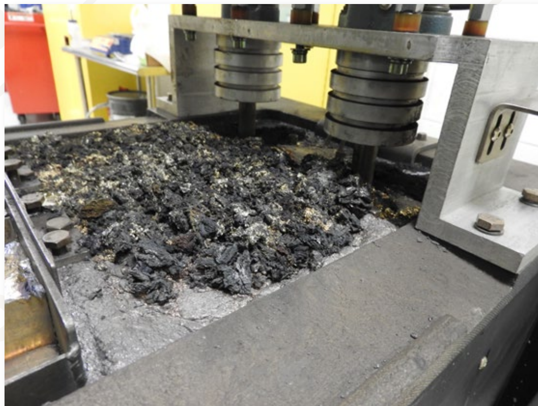
SOLDER POT WITH 1" OF DROSS
