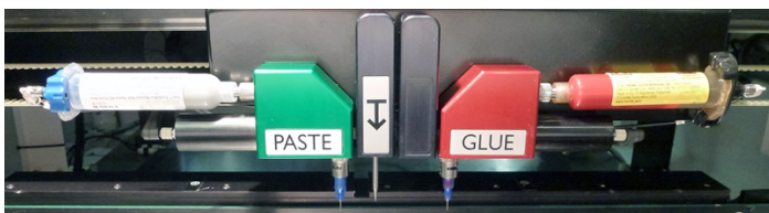
FIGURE 1. Solder paste dispenser mounted inside stencil printer.
