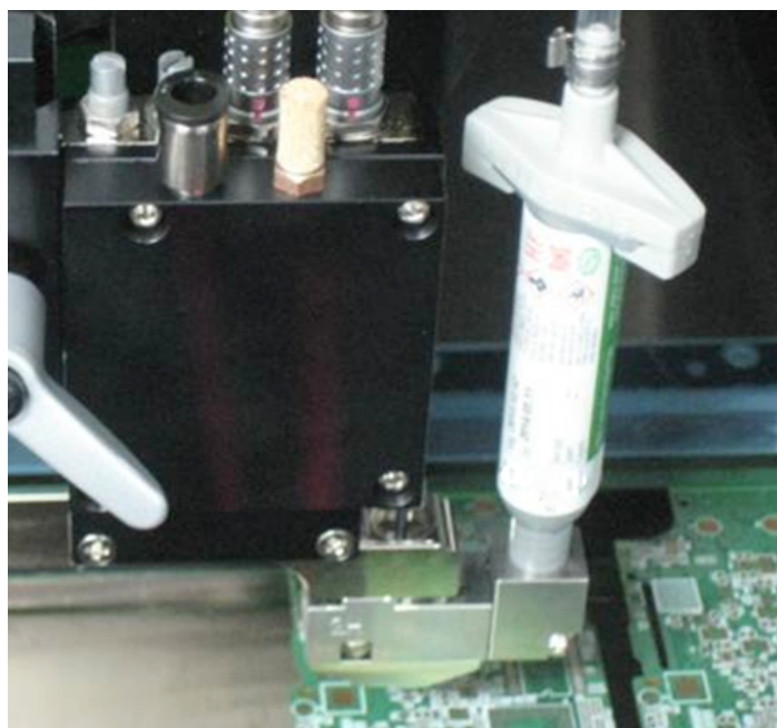
FIGURE 3. Jet dispenser on SPI system touches up insufficient paste deposits and then re-inspects to assure proper volume.
