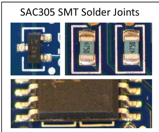
**Figure 10.** SAC305 solder joints formed in Case 1.
