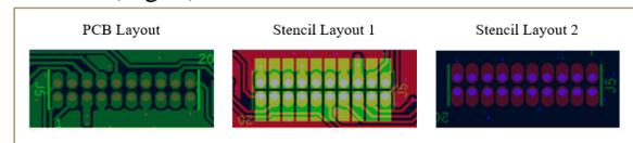
Figure 1. PCB and stencil designs for Phase 1 of DOE.
