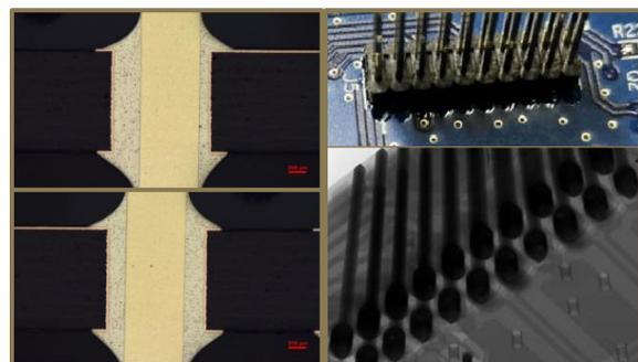
Figure 2. RTS profile produced IPC-610G compliant solder joints with full barrel fill and minimal voids on PiP components.
