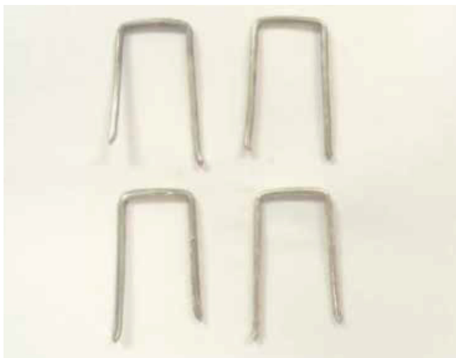
FIGURE 1. Tin whisker test specimens.
