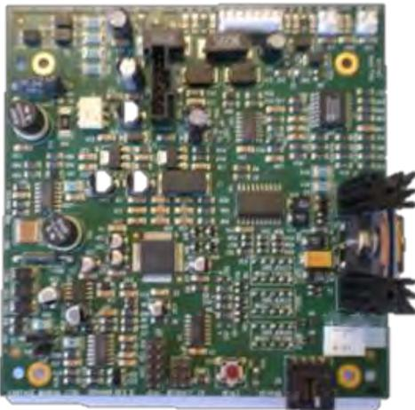
**Figure 2.** Controller board used in baseline production run (Case 2/PCB 2).
