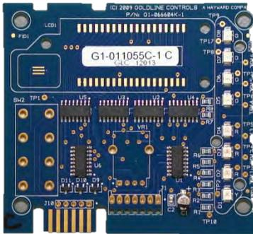
**Figure 1b.** Display board used in experimental production run (Case 1b/PCB 1b).
